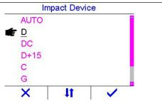
Make sure the selected or the automatically identified impacted device agrees with the connected one.
