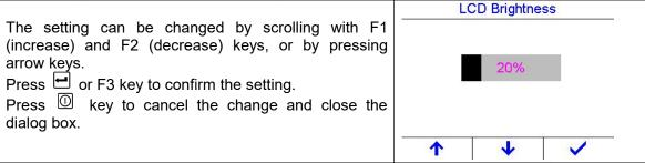
The instrument consumes less current in lower brightness and consequently increases the operating time.
