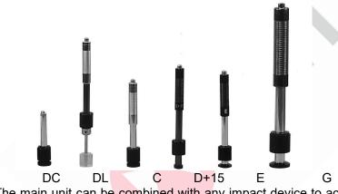
The main unit can be combined with any impact device to accommodate specific needs. Special impact devices are available for use in confined spaces, with special component geometry or surface finish.
