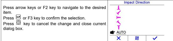
If AUTO item is selected, the impact direction will be detected according to the rebound signal of the impact body and the measurement value will be corrected automatically by the main unit. **Note:**
