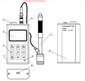
1,The main unit 2,Keypad 5,Socket of impact device 8, Label 9, USB port
